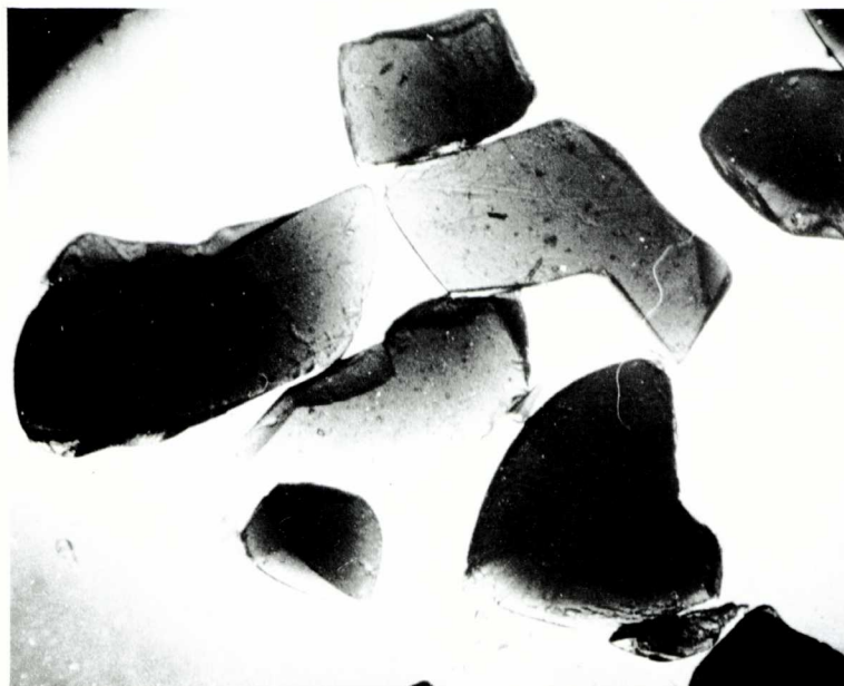
Fig. 2. The single crystals from ultracentrifuge precipitate (PVC-I).
